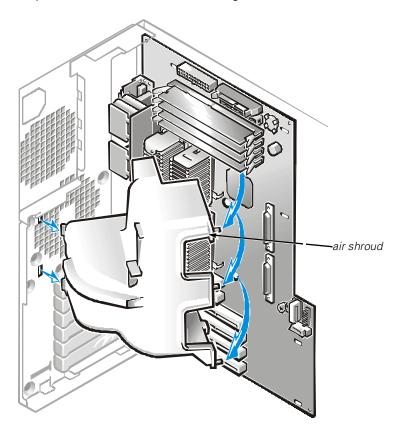
Figure 8-8. Removing Air Shroud
